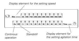
The basic model of the device can be used in continuous or timed mode depending on the option you select. The right turn button is used to make the setting.
